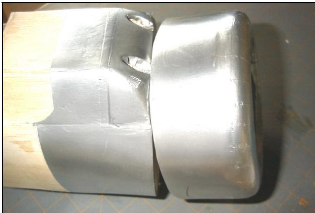
A simple cowl fixing may be made by making two L shaped brackets from scrap material. The top of the rearmost C1 hooks into them, and two small screws retain the bottom. Screwdriver access is through the open front of the cowl.
