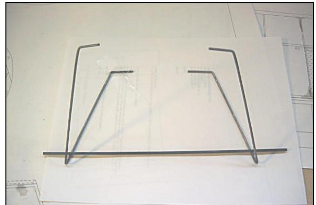
Bind the undercarriage wires to formers F4 and F5, bind and solder the wires to the axle and then glue the top bindings. Alternatively, the u/c may be retained using saddle clamps and screws
